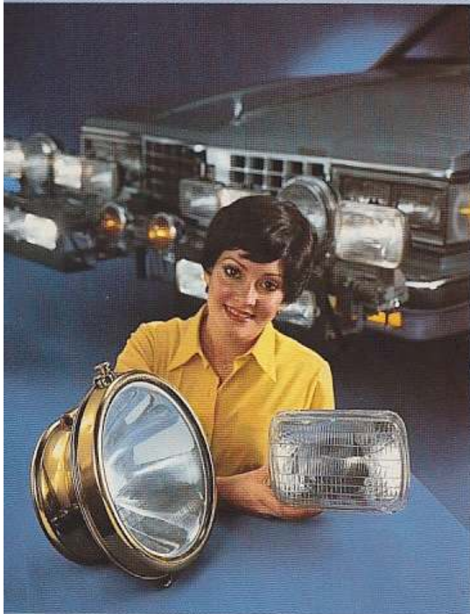
The first electric headlamp produced by Guide in 1908, compared with a modern tungsten-halogen sealed beam unit. Test car, used to evaluate lighting systems, appears in background.
