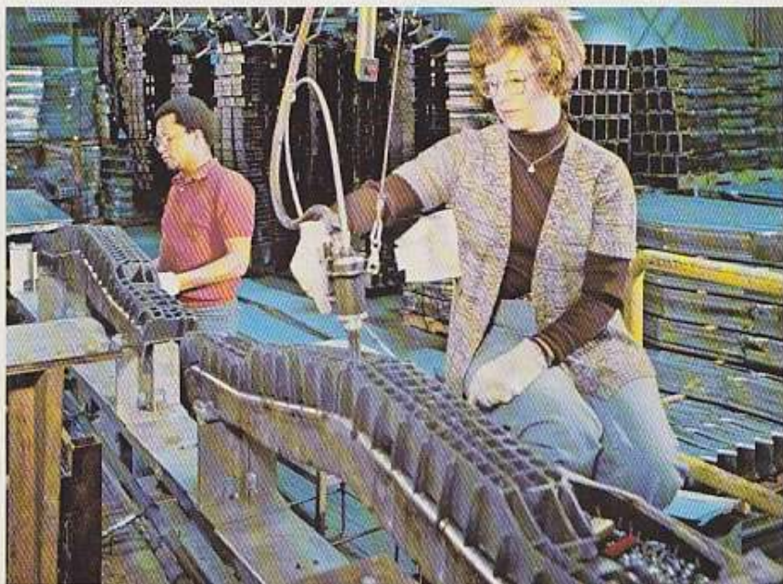
Fig 5. In first subassembly step, energy absorber is fastened to metal support bar using Pop-type rivets. Support bar may be stamped from steel or aluminum. This subassembly serves the same function as the hydraulic cylinders and mounting brackets of conventional bumper systems weighing about twice as much.
