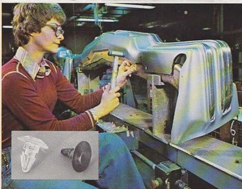
Fig 7. And finally, at adjacent station, the fascia is permanently attached to the energy-absorber subassembly. Polycarbonate snap-in fasteners (see inset) secure fascia to bottom edge of bumper-support bar. Pop-type fasteners are used to secure the top edge. The Guide-Flex bumper is now completed, ready for shipment.
