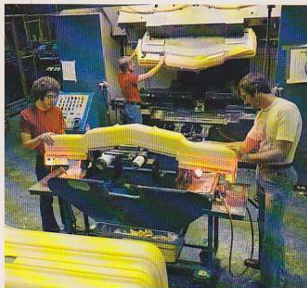
Reaction injection molding operators Steve Long, left, and Bruce Hatfield trim a plastic Guide-Flex bumper fascia, as operator Roger Cuneo removes another fascia from the molding machine.
