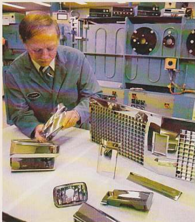
Senior project engineer Canby Willson demonstrates the flexibility of "sputtered" chrome plating on an experimental plastic part. New, innovative method of chrome plating, developed by Guide, may revolutionize the finish of flexible injection molded components.
