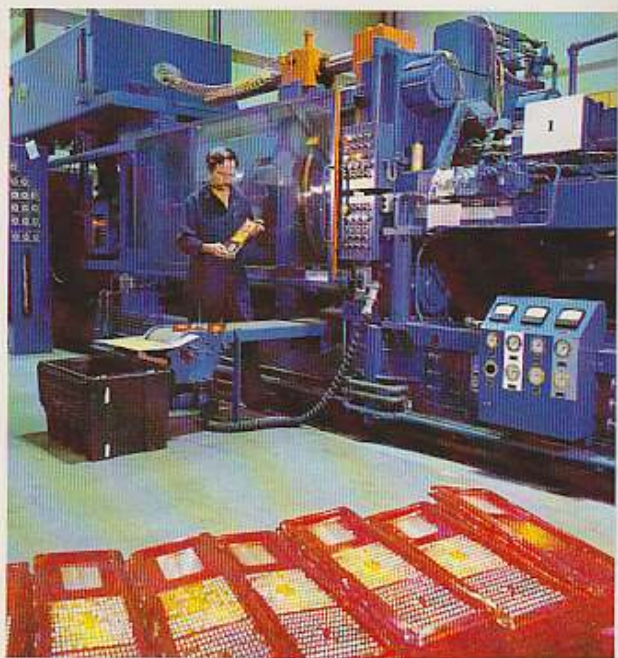
Die setter King Huntzinger examines a plastic lens for an auto tail lamp, similar to those in foreground. The three-color lens is molded in one piece in this big injection molding machine.
