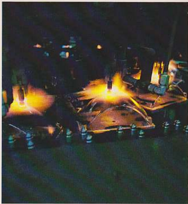
In this headlamp manufacturing process, gas-fed flames at a temperature of 2,300 degrees Fahrenheit are used to seal metal ferrules into the glass reflectors of sealed beam units. The ferrules seal openings in the reflectors and provide means of making electrical contact to the filaments.
