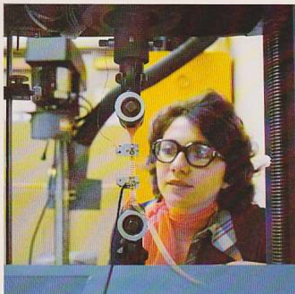
A sample piece of reaction injection molded bumper fascia is given a test for tensile strength and elongation by project engineer Rachel Layton.
